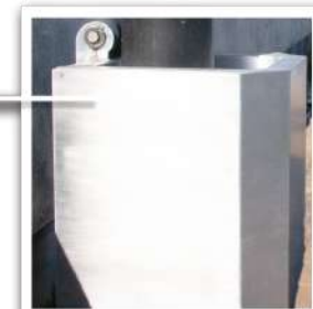
Protective Cowling Constructed with 6061-T6 Aluminum
